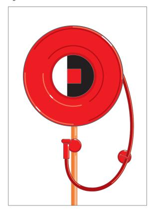
Maintenance of hose reels includes visual checks for leaks and obvious damage, which should be carried out regularly. A competent person should carry out more formal maintenance checks at least annually.
