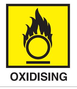
Figure 7: Label on oxidising materials
